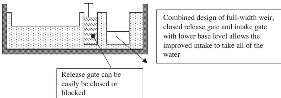
Fig. 4 . Improved intake – end view.
