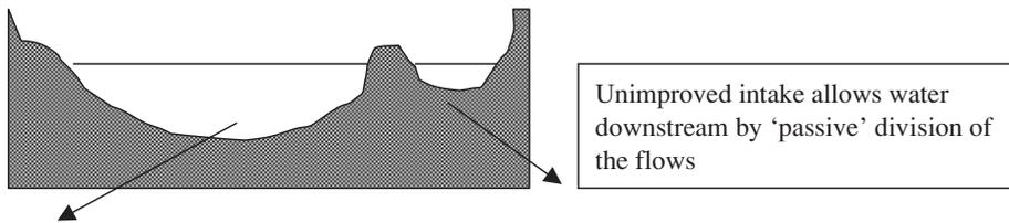
Fig. 3. Unimproved intake – end view.
